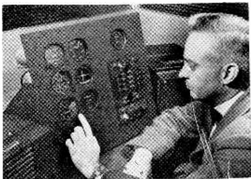
Airborne Equipment. This panel displays all the instruments and messages necessary for complete operation of the Data Link on board an aircraft. The operator is pointing out the bearing indicator,
